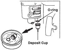
5. Push the Gas Valve to the open (right) position and check for gas leaks from the Deposit Cup. Reinstall the Deposit Cup and tighten hardware.
